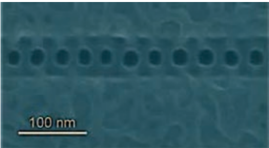
Silicon nanoparticles row deposited onto a nanotrench defined by means of graphoepitaxy.
