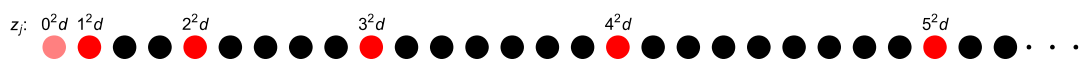
Fig.1: Schematic diagram of the Gauss chain. z_j = j^2d labels positions of lattice sites (pink for j = 0 , red for j \in \mathbb{N} ). The atomic form factor of the sites in black is zero. The Fourier transform of this chain is the Jacobi theta function \theta_3(q) with q = \exp[i(k + i\alpha)d] the nome and \alpha \rightarrow 0 a convergence factor leading to a highly complex structure factor despite the chain's simplicity.
