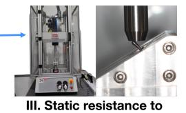
fracture tests (ISO 14801:201). .
