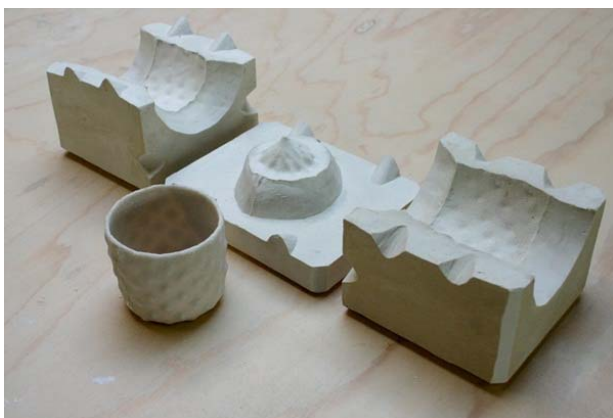
Figure 10 Intermediate results of the 17 th century glass reproduction (plaster mold and 3D print).
